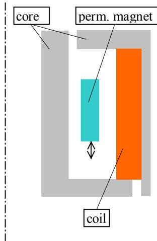
**Fig.6** – Principal construction of the moving magnet actuator
