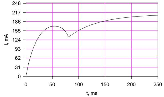
**Fig.2 – Solenoid actuator – coil current**
