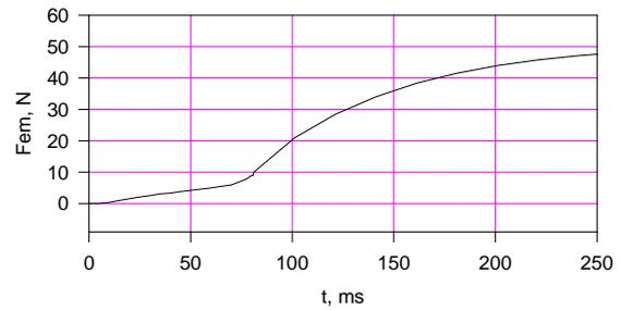
**Fig.3 – Solenoid actuator – electromagnetic force**
