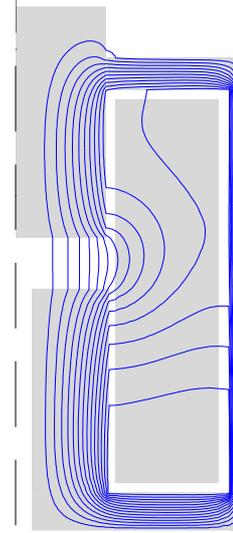
**Fig.1 – Solenoid actuator with static field plot**
