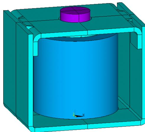
**Fig.16** – Driving electromagnet of DC contactor
