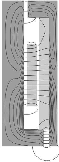
**Fig.9** – Moving magnet actuator - field plot at  $t = 435 \text{ ms}$
