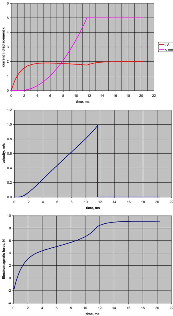
**Fig.14** – Bistable actuator- results
