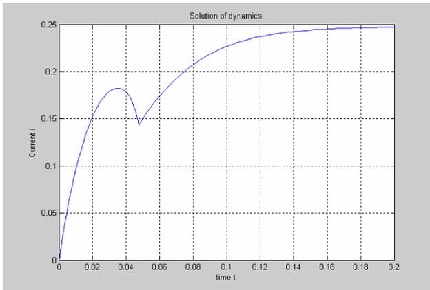
**Fig.17** – DC contactor- coil current
