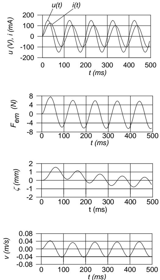
**Fig.8** – Moving magnet actuator - voltage  $u$ , current  $i$ , electromagnetic force  $F_{em}$ , displacement  $\zeta$  and velocity  $v$  versus time  $t$  at 10 Hz frequency
