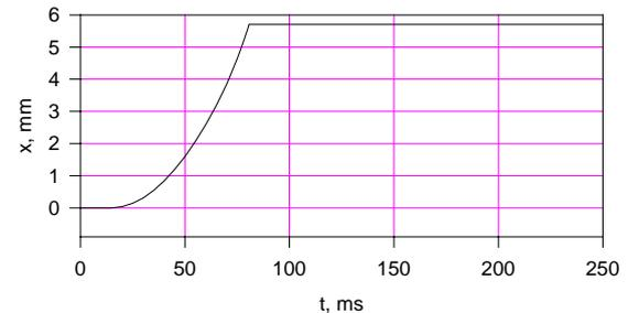
**Fig.4 – Solenoid actuator - displacement**
