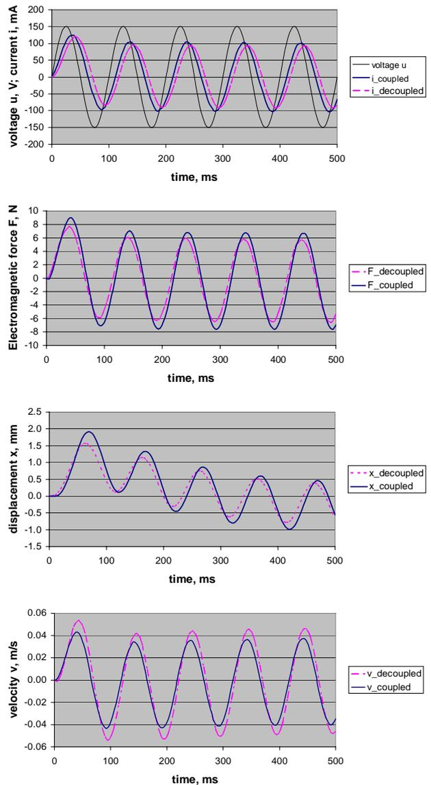
**Fig.15** – Moving magnet actuator – results using coupled and decoupled approach
