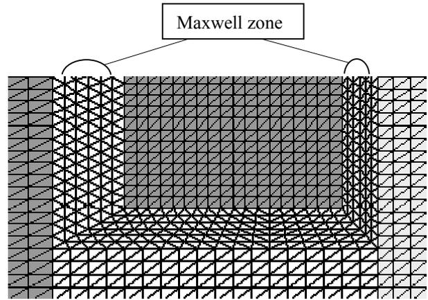
**Fig.7** – Fragment of the mesh near the lower part of the permanent magnet
