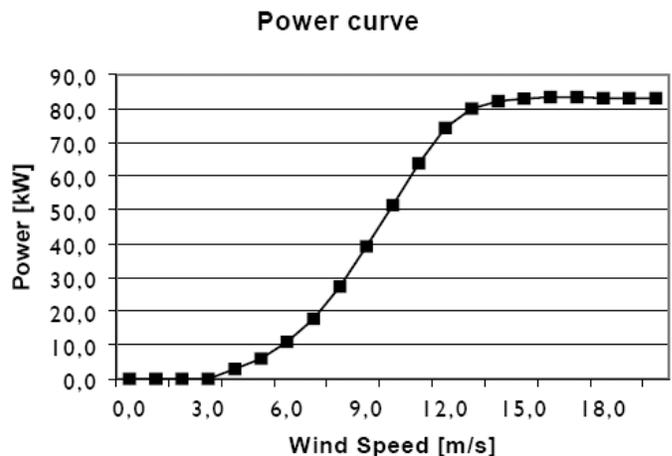
Fig.5. Power curve of Lagerwey 18/80
