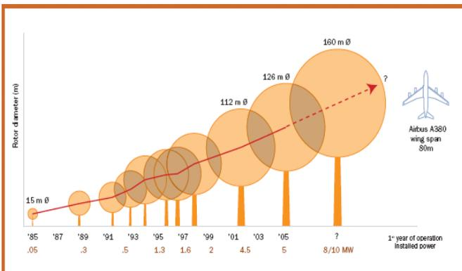
Fig. 2. The size progression of wind turbines. Mid 2005 the largest wind turbine had a diameter of 126 meters and an installed power of 5 MW [6].
