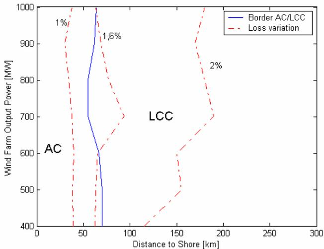
Fig.4. “MW-km” plane, comparison HVAC-HVDC LCC for different wind farm size (400-1000 MW) and different distances to shore (0-300 km) for average wind speed of 9 m/s [14].
