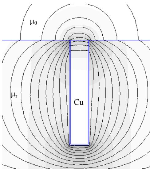
**Fig. 1** – Field lines in the surrounding of rectangular cross-section conductor in the groove of ferromagnetic block
