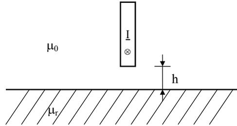
Fig. 2 - Conductor with the current  $I$  in the ferromagnetic surrounding
