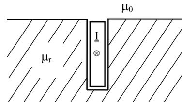
Fig.4 - Rectangular conductor in the ferromagnetic block groove
