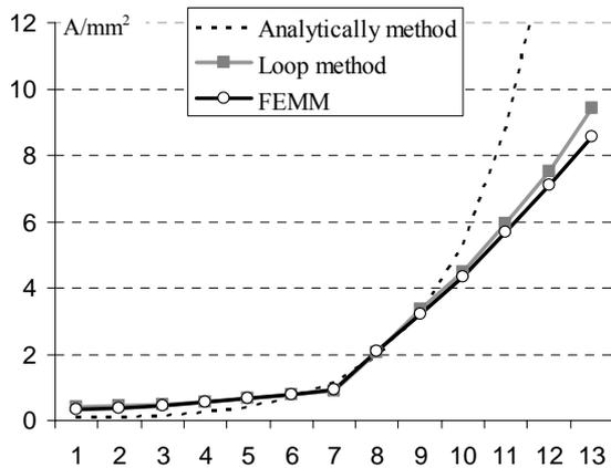
**Fig. 9** - Graph illustrating the results of calculating current density along conductor vertical axis
