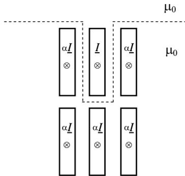
**Fig.5** - The influence of ferromagnetic surrounding replaced with the equivalent currents in the homogenous surrounding
