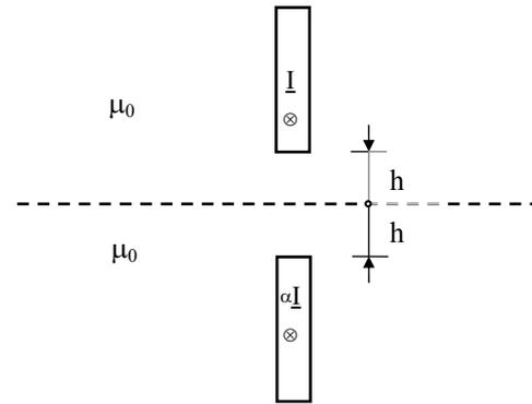
Fig.3 - Conductor with the current  $I$  and its image
