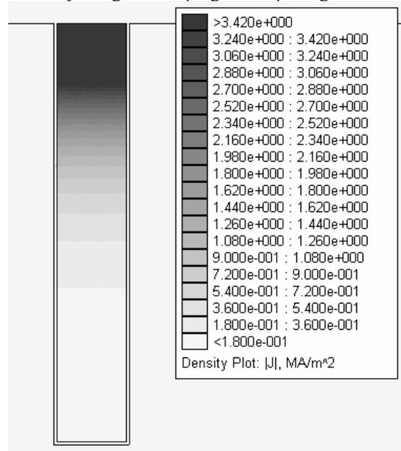
**Fig. 8** - Distribution of current density obtained by applying FEMM programme package
