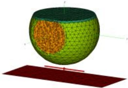
**Fig.4** – FEM/MoM: Hybrid MoM/FEM with full coupling between the MoM and the FEM.
