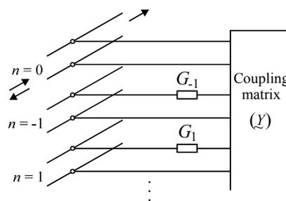
Fig.2 - Equivalent network model for the problem from Fig.1
