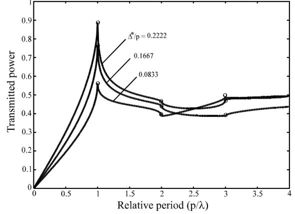
**Fig.3** - The relative transmitted power of the basic mode versus the relative period  $p/\lambda$  for the TE polarization. Parameters from Fig.1 are  $d^*/p = 0.5$ ,  $d_1^*/p = 0.02776$  and  $\theta = 0^\circ$ .
