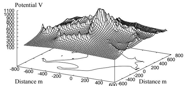
Fig. 4 - Calculated values of the potential distribution around the 110/10 kV substation
