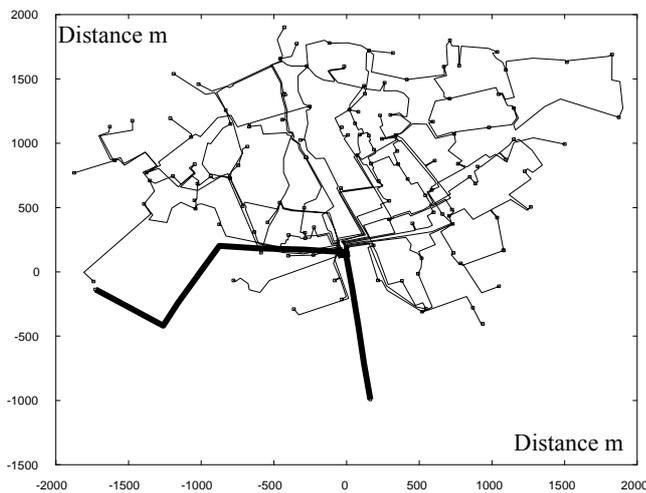
Fig. 3 - Grounding system connected to cable network of existing 110/10 kV substation in urban area
