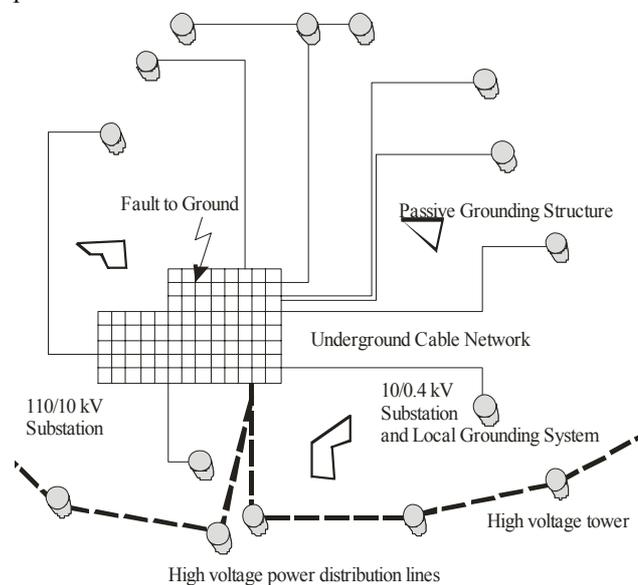
**Fig. 1 - Grounding system of high voltage substation connected to underground cable network**
