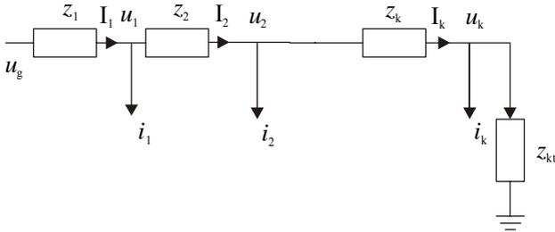
Fig. 2 - Equivalent circuit of the uncoated metallic sheathed cable
