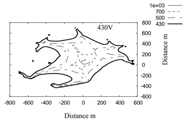
Fig. 5 - Calculated equipotential lines around the 110/10 kV substation and the limit according to the CCITT directives
