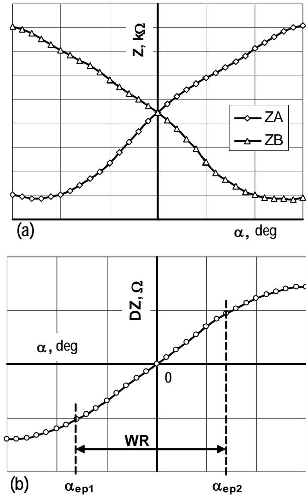
Fig. 2. - The dependence of the impedances to the angular displacement  $\alpha$
