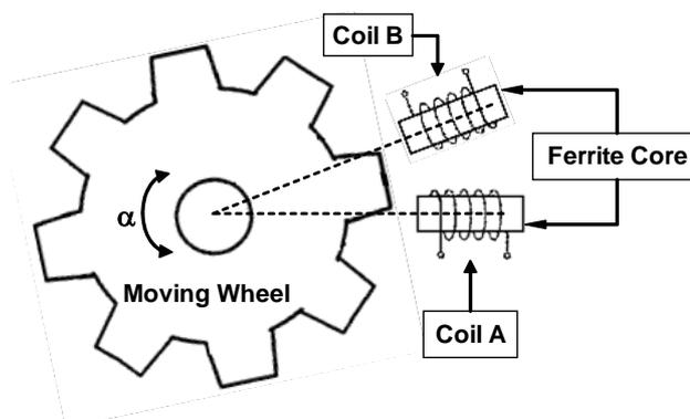
Fig. 1. - The Inductive Transducer
