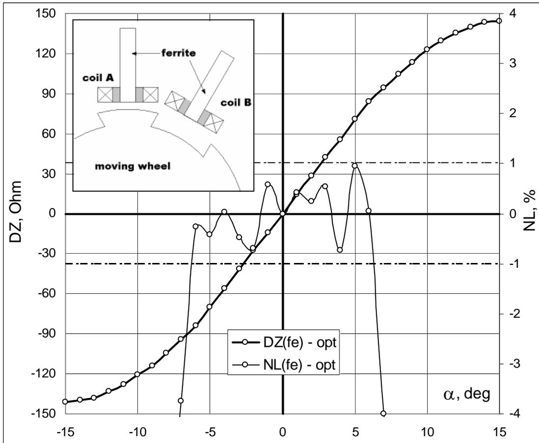
Fig. 4. - Ferrite cored DIT - transfer function and linearity characteristics
