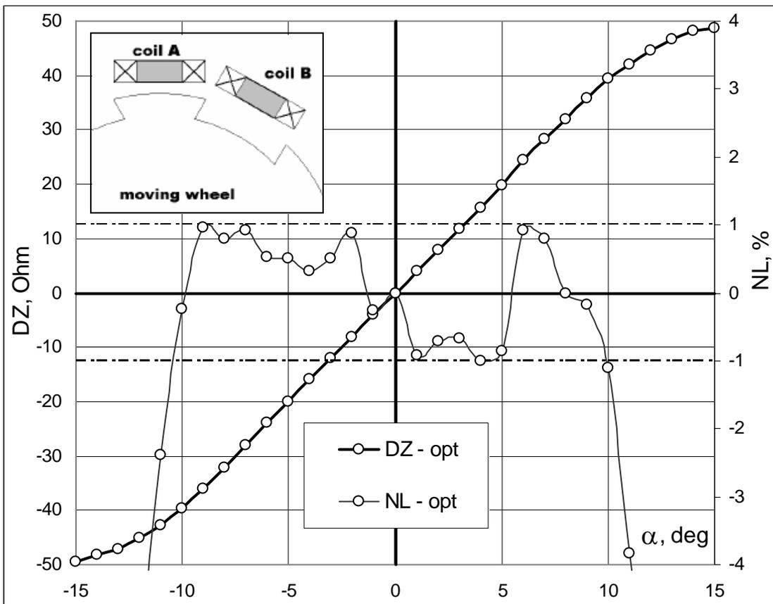
**Fig. 5. - Air cored DIT - transfer function and linearity characteristic**
