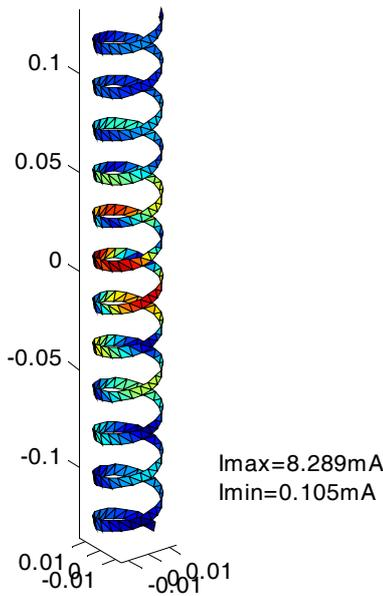
Fig.2- Current distributions and maximum/minimum current of helical antenna
