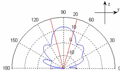
Fig.6. – Radiation pattern 14-turns axial mode helical antenna
