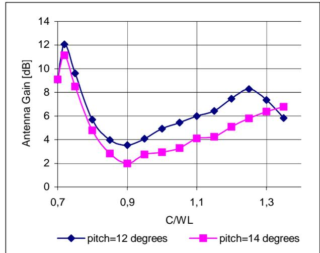
Fig.3 - Helical antenna gain vs. pitch angles and circumference
