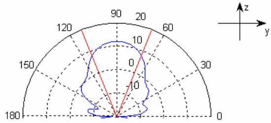
Fig. 5. – Radiation pattern 12-turn helical axial mode helical antenna at 2.4GHz
