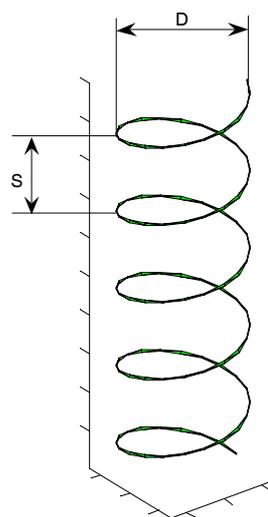
Fig.1 – Helical antenna geometry
