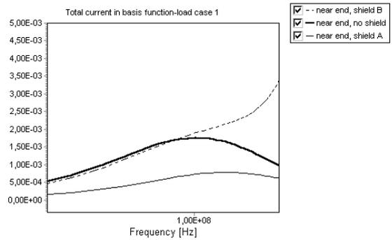
**Fig. 12.** Near end crosstalk - shield A versus shield B, load case 1,  $f=(10-350)$ MHz
