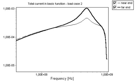
Fig. 7. Near end and far end crosstalk for load case 2
