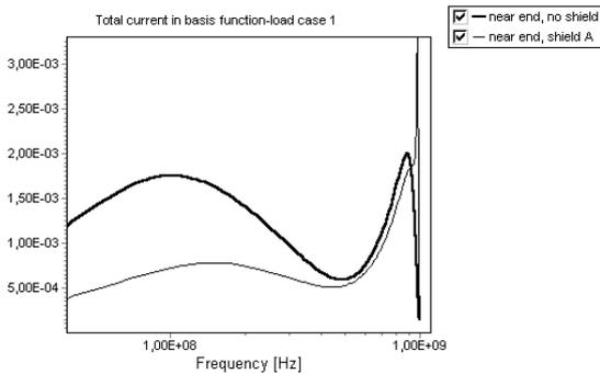
**Fig. 10.** Near end crosstalk with and without grounded shield for load case 1
