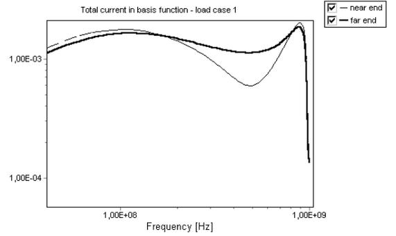
Fig. 6. Near end and far end crosstalk for load case 1
