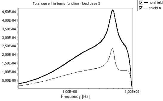
**Fig. 13.** Near end crosstalk with and without grounded shield for load case 2
