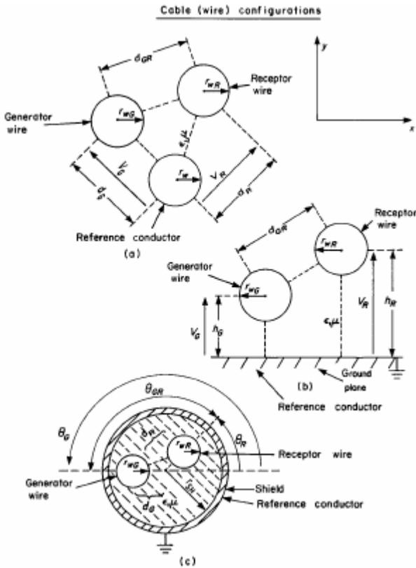
**Fig. 3.** Wire-type line cross sections whose reference conductors are (a) another wire, (b) an infinite ground plane, or (c) an overall, cylindrical shield
