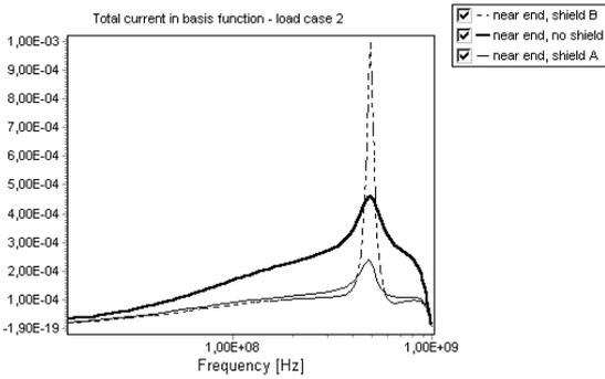
**Fig. 14.** Near end crosstalk - shield A versus shield B, load case 2,  $f=(10-1000)MHz$
