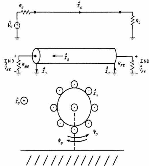
Fig. 9. Illustration of the effect of placing a shield around a receptor wire on inductive coupling
