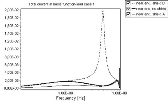
**Fig. 11.** Near end crosstalk - shield A versus shield B, load case 1,  $f=(10-1000)$ MHz
