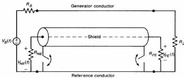
Fig. 8. Shield around the receptor circuit wire to reduce crosstalk
