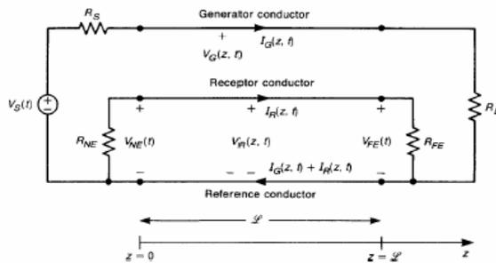
Fig. 2. The general three-conductor transmission line, illustrating crosstalk
