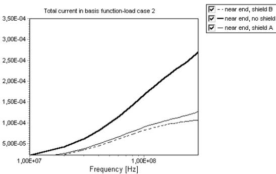
**Fig. 15.** Near end crosstalk - shield A versus shield B, load case 2,  $f=(10-350)MHz$
