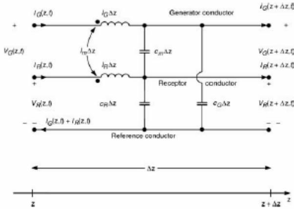
Fig. 4. The per unit-length equivalent circuit of a three-conductor transmission line
