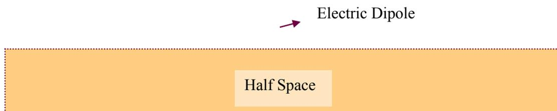
Fig. 2: A dipole over a half space. The problem was first solved by Sommerfeld to understand the propagation of radio waves over the lossy earth.
