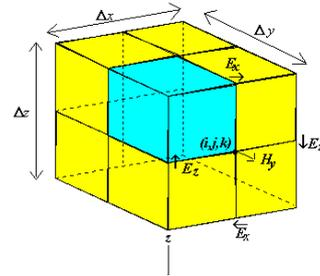
Fig. 4: Description of field quantities on a rectangular 3D grid (YEE cell)
