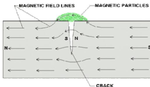
Fig.2 - Localization of particles around the crack [3]
