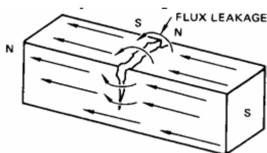
Fig.1 - Magnetic leakage around crack [3]
