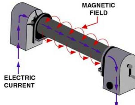
Fig.5 – Direct magnetization [3]
