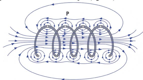
Fig.7 – Magnetic field of a solenoid [3]
