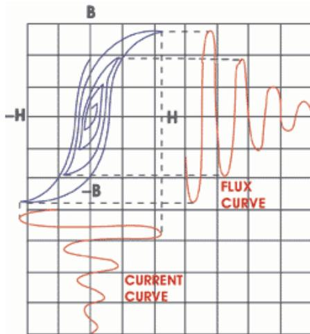
**Fig.8** – slowly reducing AC current used for demagnetization [3]
