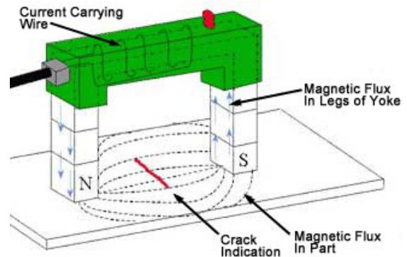
Fig.6 – Indirect magnetization [3]
